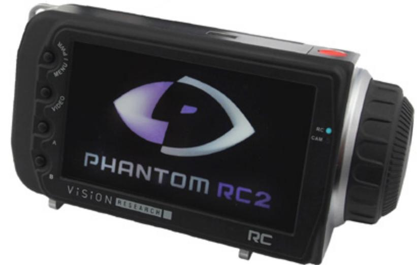
The Phantom Remote Control Unit (RCU) is a small, lightweight, hand-held controller which allows you to adjust most settings on your camera as well as view and save recorded cines to the CineMag IV. The RCU is available in both wired and wireless versions. Both versions will connect with an included 5 meter cable direct to the back of the camera. Alternatively, the wireless model includes a Bluetooth dongle that allows for operation from up to 100 meters.
