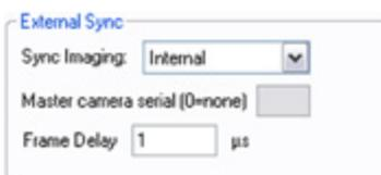
'External Sync' instructs the camera to utilize one of the following three frame sync clock sources:
